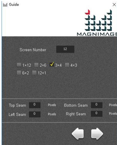
No. of screens can be set here, namely: number of output port. Take 12 as an example, set the screen number as 12, several kinds of combination will be offered (No. of row x No. of column, eg. 3x4 means 3 row x 4 column). Select proper combination, and convert the seam of LCD into pixels, fill in the seam table below, click next, the software will build output screen automatically, as shown in below image.
